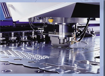
9 Station w/300° Rotation Punch Press with the Ability to Hold 90 Tools Including Forming and Tapping Tooling.
